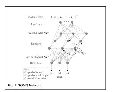
The input layer takes the sensory input as the input to the layer. This represents the state of the robot in the environment. The next layer is rule layer that map the input state of the robot to the possible actions of the robot. This layer is a layer of nonlinear units that are connected to all the nodes in the input layer.
