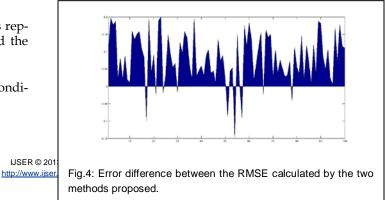
The error difference of the two networks is calculated and plotted against the number of iterations. As can be seen, the error is significantly reduced by including the localization factor in the input.
